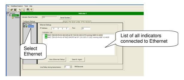
Once Ethernet is selected, the Ethernet settings window will be opened. A list of all available Ethernet connections to indicators is in the main window
