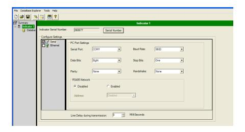
If the USB port is connected to the serial port, and an OVERRUN error occurs, change the Line Delay to 50ms or 100ms. This will slow down the information passing from Wedge to the indicator.
