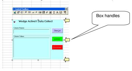
When the control has focus, you should be able to click on the **Properties** button (the finger pointing to the page) and the properties for the selected control should
