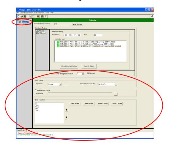
Change the parameters for the **Data Format**, the **Data Logger** and the **Data Template** as required
