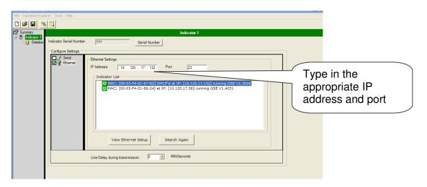
To view the Ethernet setup information about a particular indicator, click on the **View Ethernet Setup** button. The GSE Web Server website will open in a new window. The Ethernet can be verified or changed on this website.
