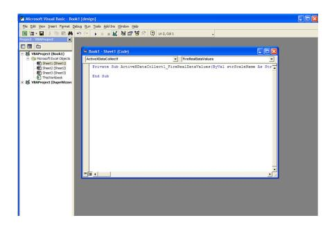
You can now write code to execute the required command. This is standard VB syntax for code written for any ActiveX control.
